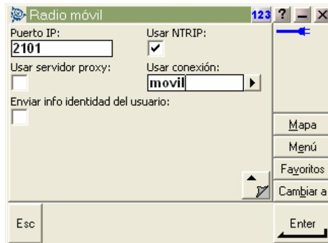
The screenshot shows the 'Radio móvil' configuration window. The 'Puerto IP:' field contains the value '2101'. The 'Usar NTRIP:' checkbox is checked. The 'Usar conexión:' dropdown is set to 'movil'. The 'Esc' and 'Enter' keys are visible at the bottom.
