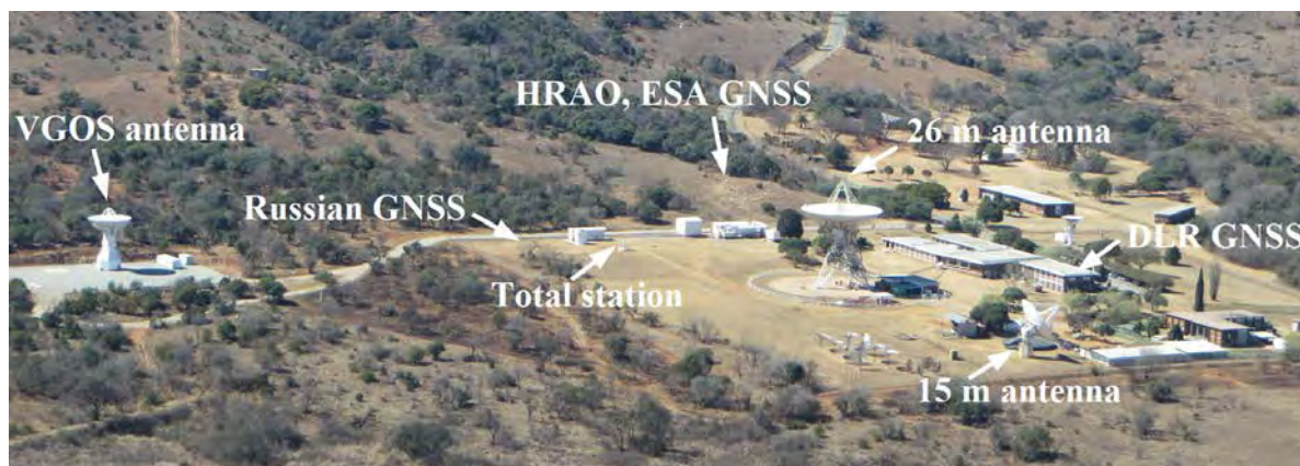
Fig. 2: VLBI local tie observing system – components of measurement and reference networks.
