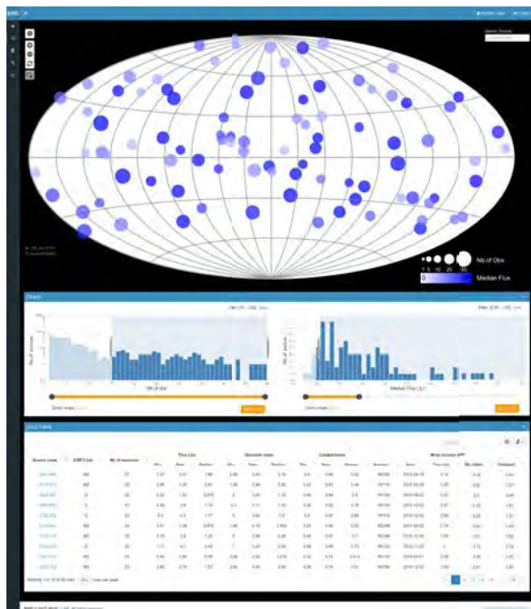
Fig. 3: View of the “Skymap” tool which allows one to display and filter sources based on the value of a given parameter (here the flux density at X-band). In this case, we selected the sources with a median flux density value larger or equal to 0.5 Jy and with a number of sessions larger than 15. This leads to a selection of 92 sources, which can be individually inspected on the sky distribution or in the source list.
