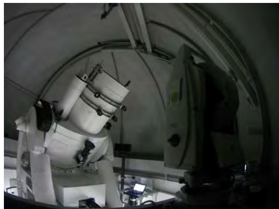
Fig. 3: Automated ILRS reference point determination of the Satellite Observing System Wettzell, using the high-precision mobile laser tracker AT401.
