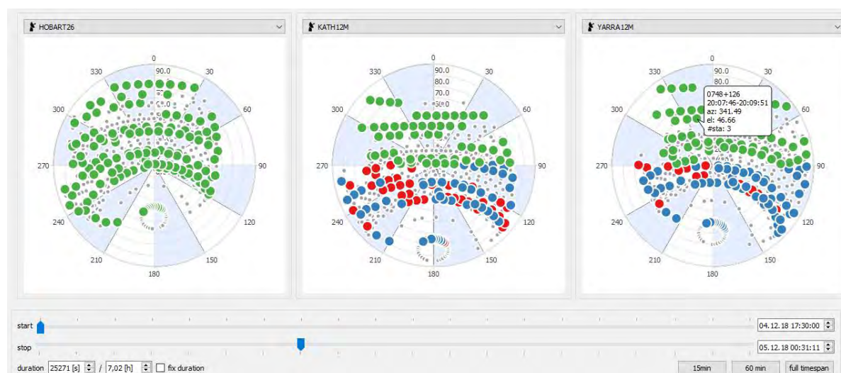
Fig. 3: VieSched++ Analyzer displaying the sky coverage of the in the session included stations, with dots representing observed sources, color-coded by the different cable wraps, counterclockwise (red), neutral (green) and clockwise (blue). The smaller grey dots represent the sources which are not observed in the selected time span.
