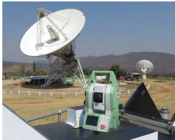
Fig. 1: Short baseline of \sim 113 m between the HartRAO 26 m antenna (left) and the HartRAO 15 m antenna (right), with the Leica MS50 Multistation in the foreground.
